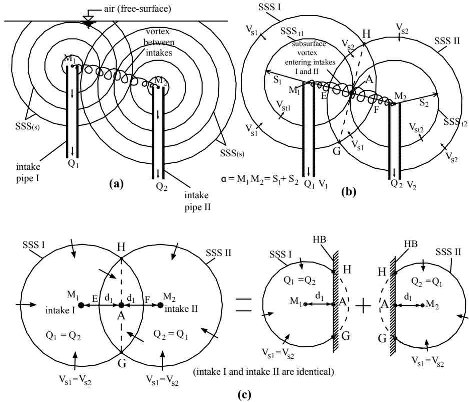
*Figure 3- (a) and (b) Subsurface-Vortex Extending between the Intakes I and II and the Theoretical Location of "A" at the Flow-Dividing Surface. (c) Imaginary Impervious Boundary (IIB) Between the Identical Intakes I and II.*
