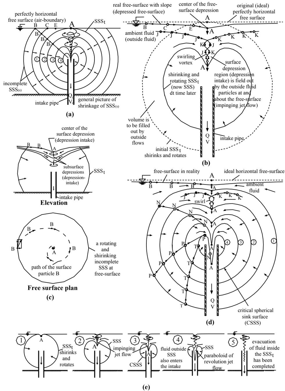
Figure 1- (a)-(e) Collapsing Stages of SSS(s) and Development of the Free-Surface Vortex Originating from the Air-Boundary.
