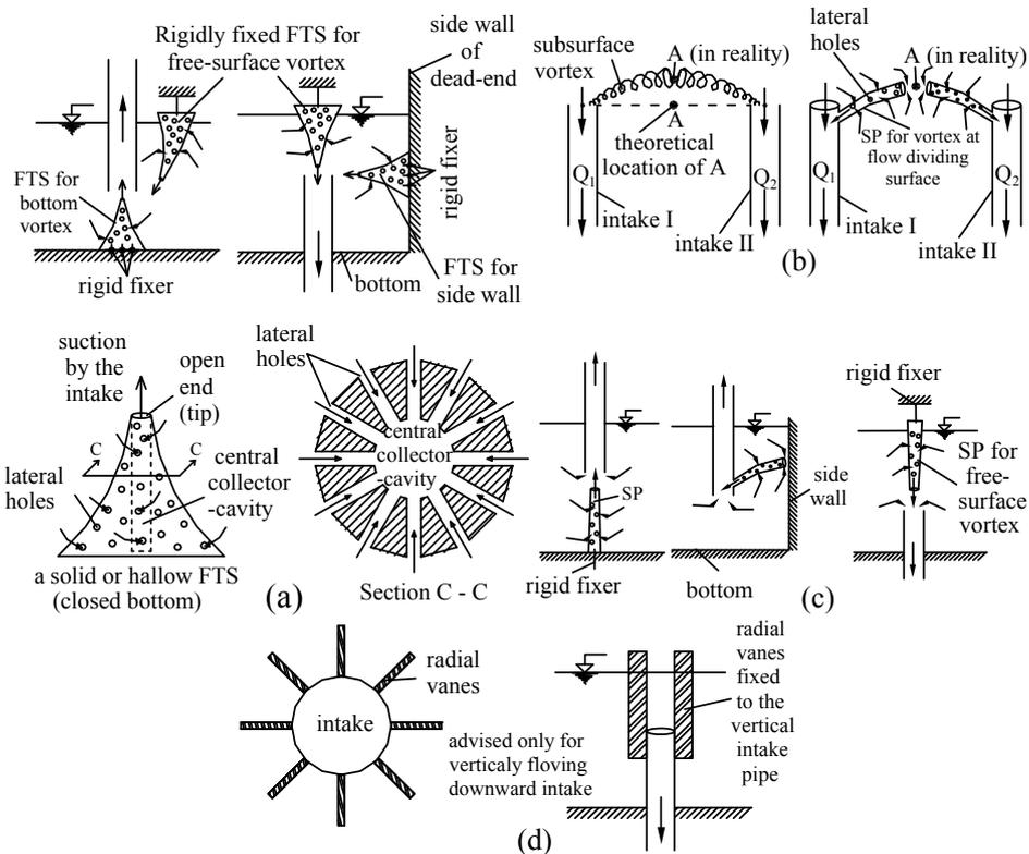
Figure 5- FTS and SP for the Elimination of Subsurface-Vortices.
