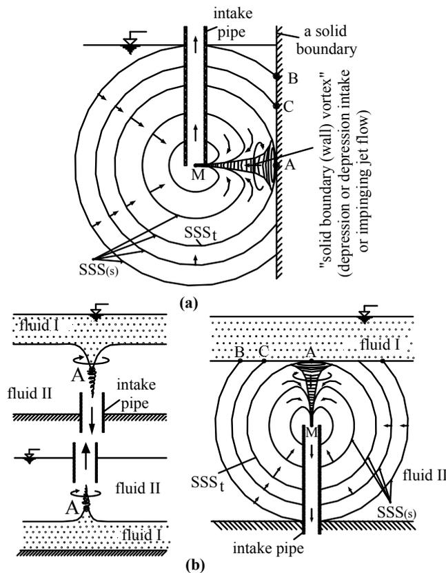
*Figure.2- Development of Vortices at (a) Solid-Boundary and (b) Stratified Fluid-Interface.*
