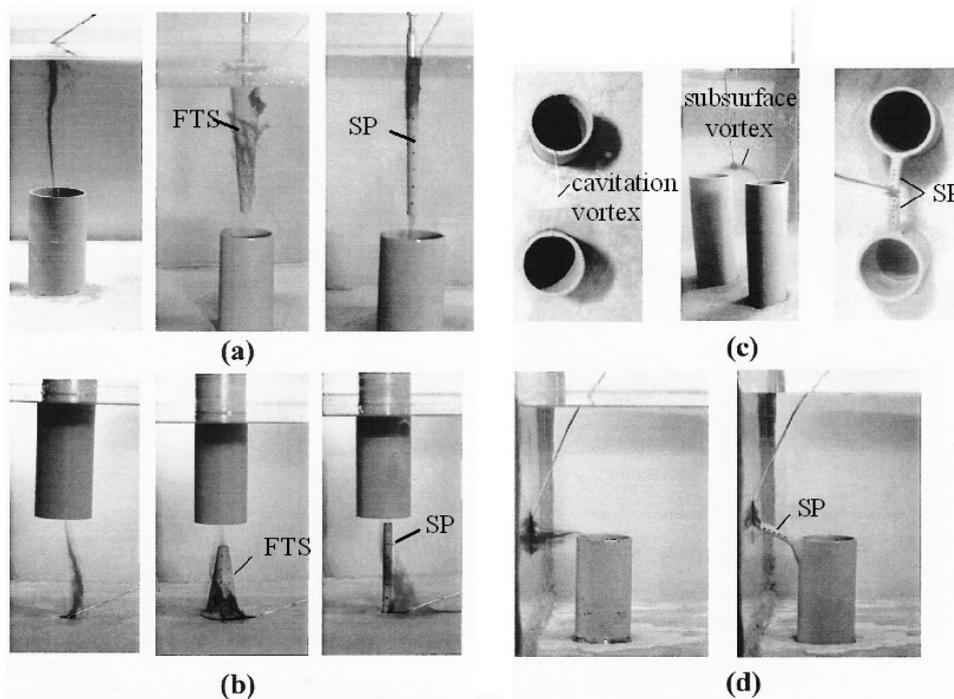
*Figure 6- Photographs of FTS and SP in Action. (a) Vertically Flowing-Downward intake, (b) Vertically Flowing-Upward intake, (c) Subsurface-Vortex Between Intakes I and II and (d) Side-Wall (Boundary) Vortex.*
