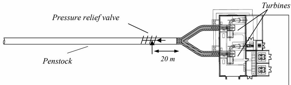
Figure 3. Plan view of the pressure relief valve and powerhouse
