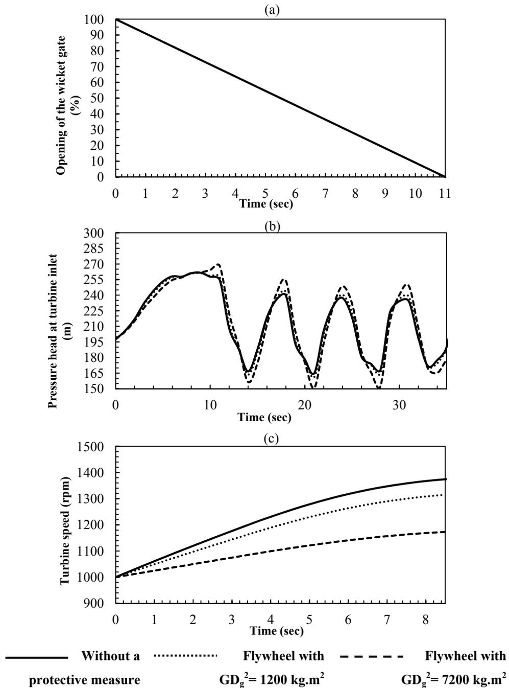
Figure 2. (a) Closure law, (b) Turbines' inlet pressure, (c) Turbines' speed rise for Scenario A
