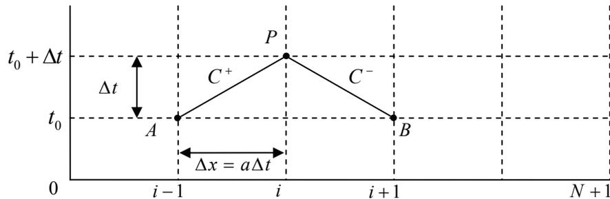
Figure 1. Characteristic lines in time-space domain
