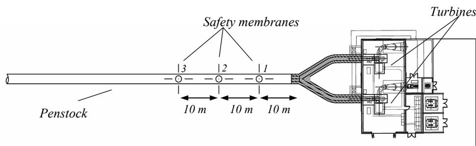
*Figure 5. Plan view of the safety membranes and powerhouse*
