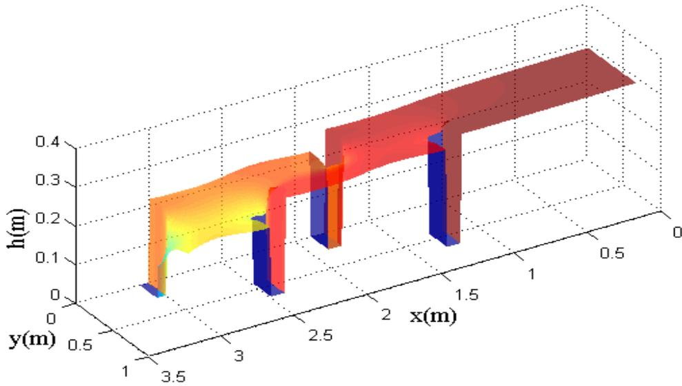
Figure 8. Numerical water surface profile through staggered spur dikes in a horizontal channel
