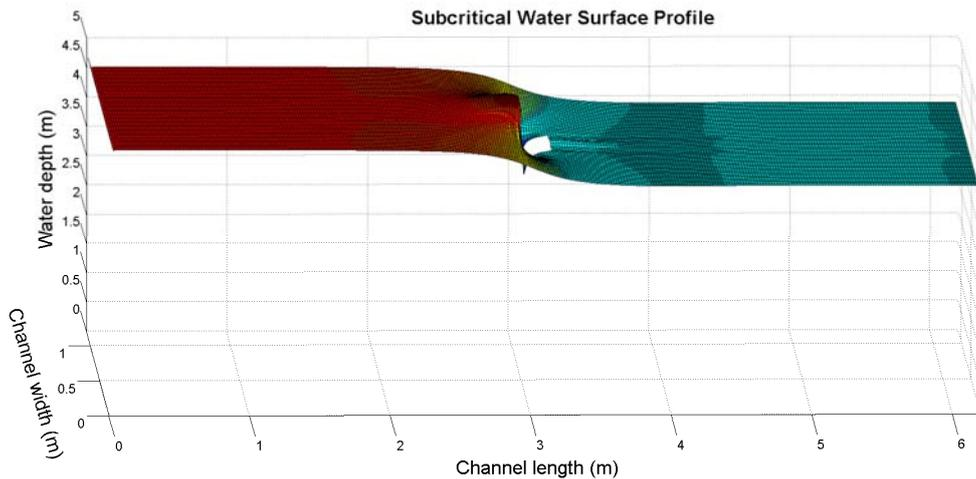
Figure 5. Water surface profile of subcritical flow around a cubic block [3]
