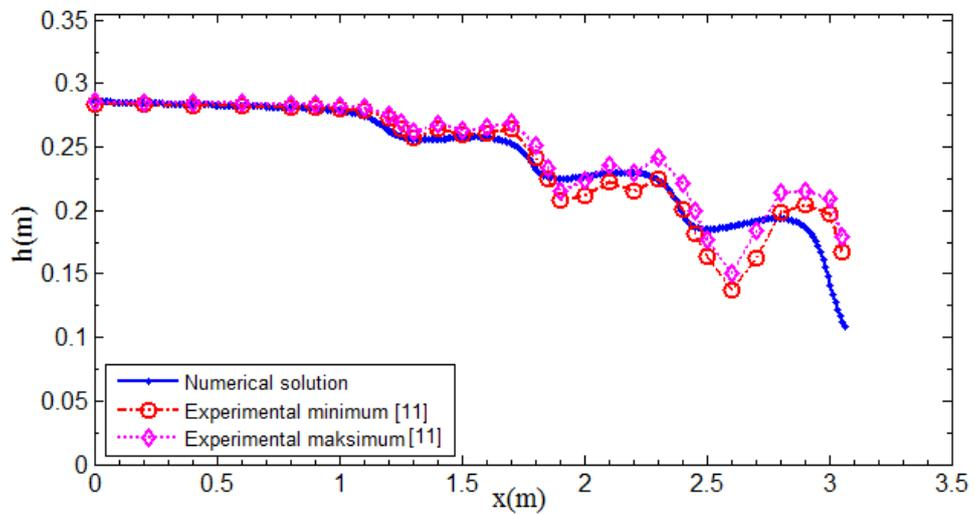
Figure 9. Comparison of experimental and numerical water surface profiles along the centerline of the channel
