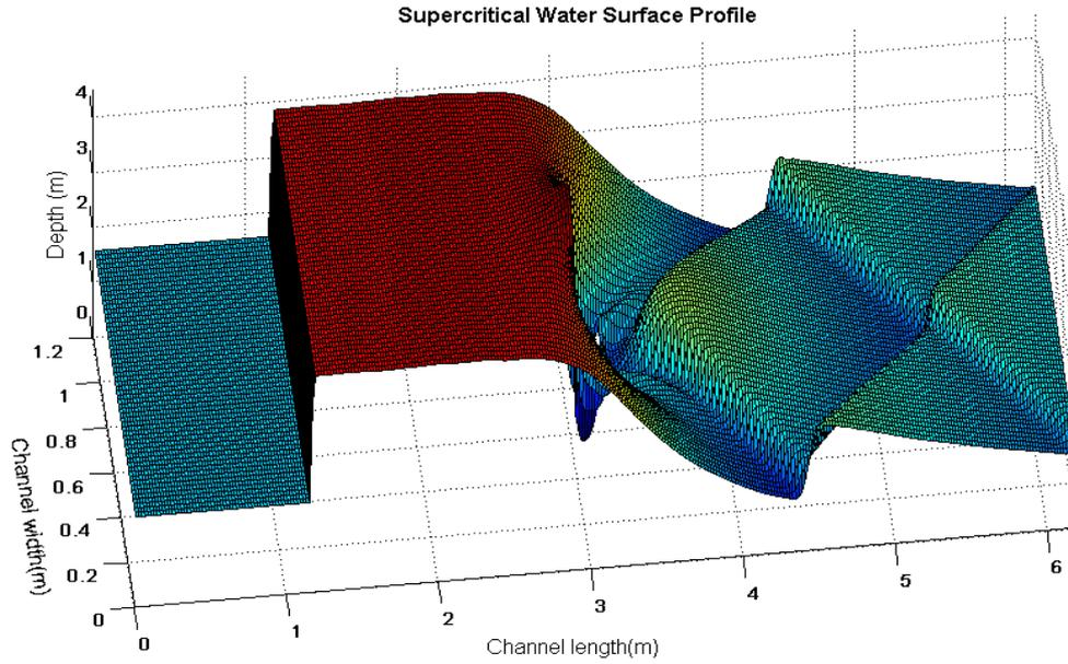
*Figure 3. Water surface profile of the supercritical flow around the cubic block [3]*
