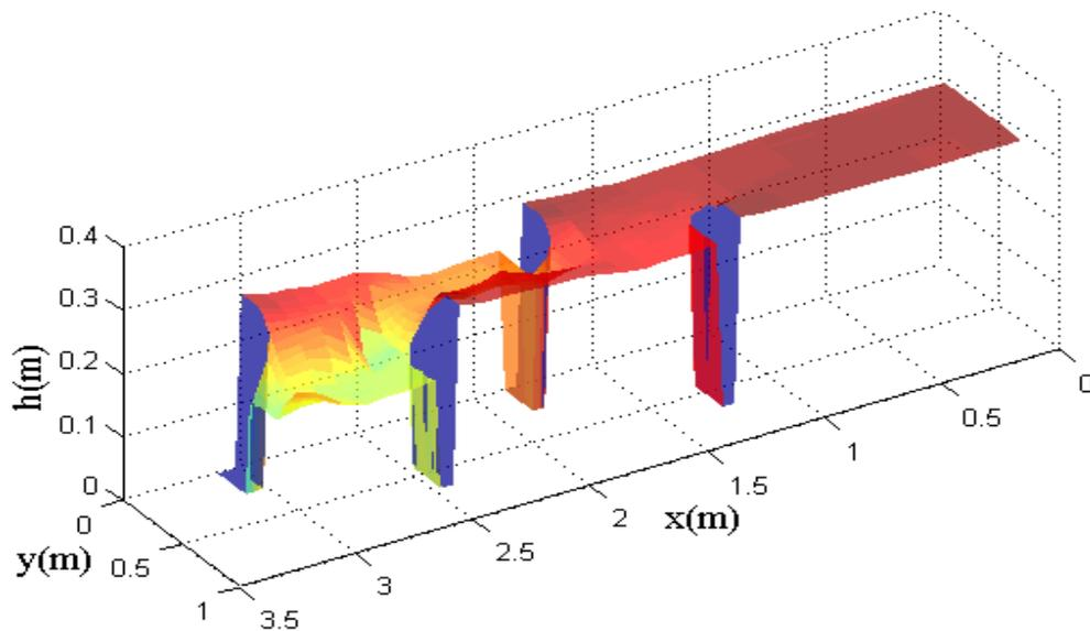
Figure 7. Experimental water surface profile through staggered spur dikes in a horizontal channel[11]
