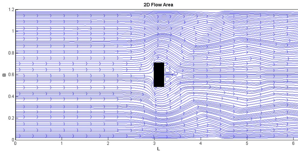
*Figure 4. Streamlines in the horizontal plane of the supercritical flow around a cubic block [3]*
