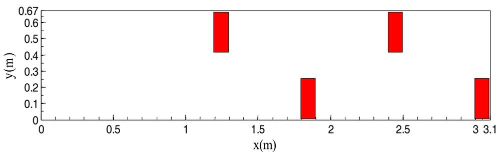
*Figure 6. Flow region in a prismatic horizontal channel with staggered spur dikes [11]*
