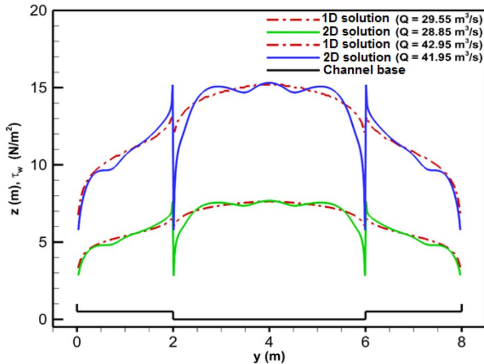
Figure 13. Comparison of wall stresses obtained from 1D SWE and 2D solutions
