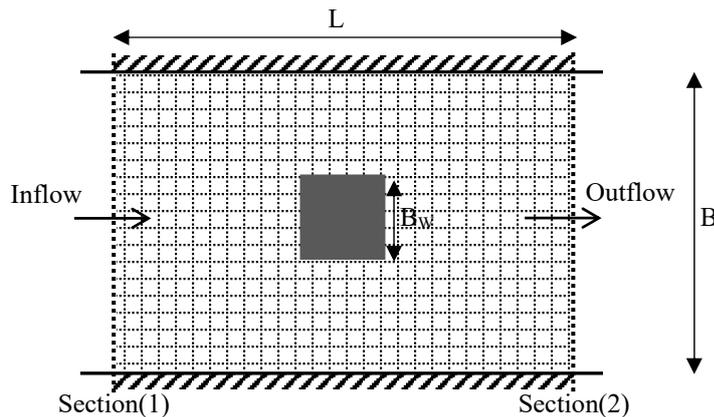
Figure 2. Numerical solution domain of the flow around a cubic block [3]
