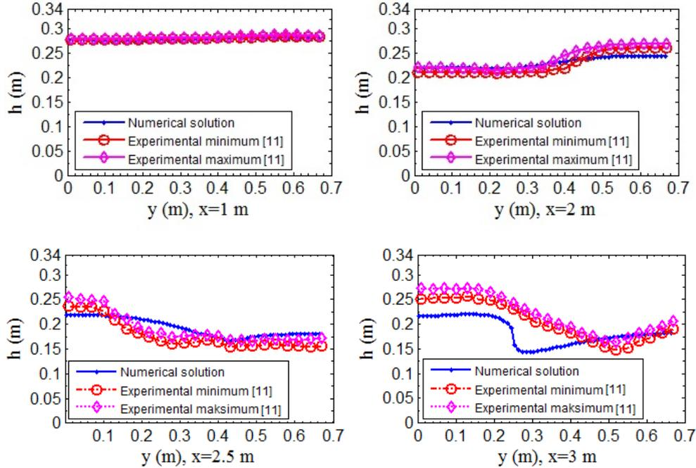
Figure 10. Comparison of experimental and numerical lateral water surface profiles on fixed channel sections
