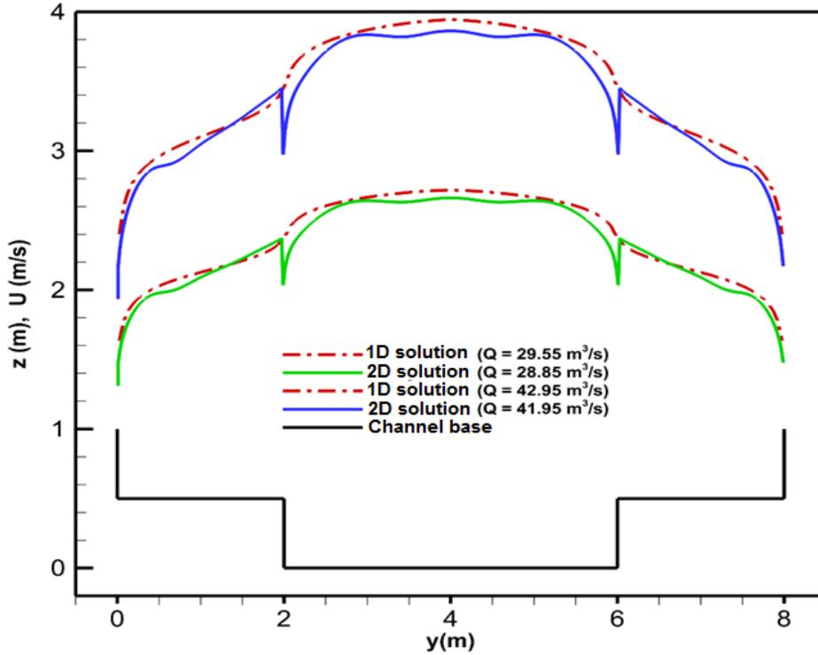
Figure 12. The comparison of depth-averaged velocities obtained from 1D SWE and 2D solutions
