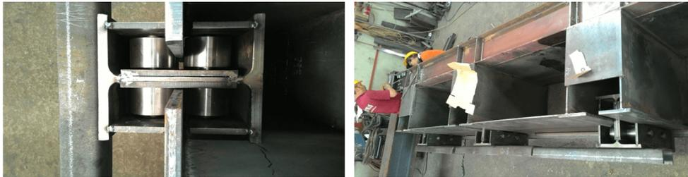
*Figure 4. Linear bearing system which is horizontally fixed, vertically free and capable to transfer moments of the connection mechanism that satisfy symmetrical boundary condition.*
