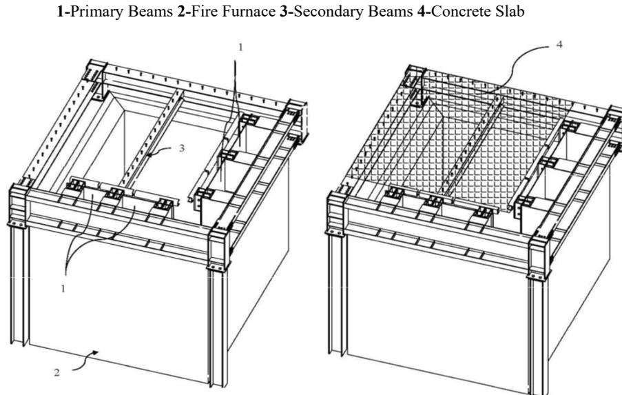
Figure 1. CAD drawings of 4.3 m x 3.8 m sized steel – concrete composite floor system on the fire furnace (a) without concrete slab, (b) with concrete slab
