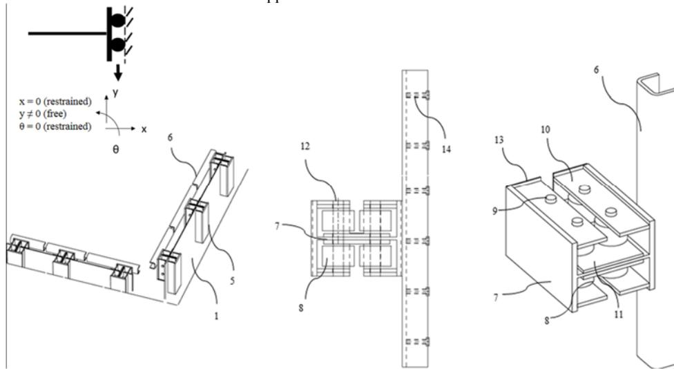
*Figure 2. Connection mechanism that satisfy symmetrical boundary conditions: CAD drawing of a linear bearing system which is horizontally fixed, vertically free and capable of transferring moments.*
