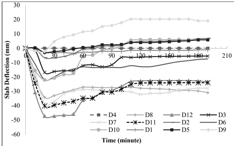
Figure 11. Slab deflections measured at different locations of the concrete slab after the static loading during the fire. (See. Figure 6)
