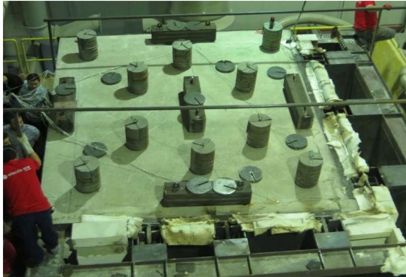
Figure 7. The loading condition on the composite floor system before the experiment.
