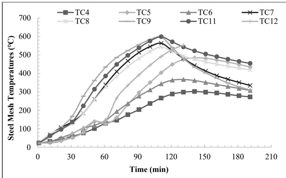
Figure 10. Thermocouple temperatures on the concrete slab steel reinforcement mesh (see Fig 5).
