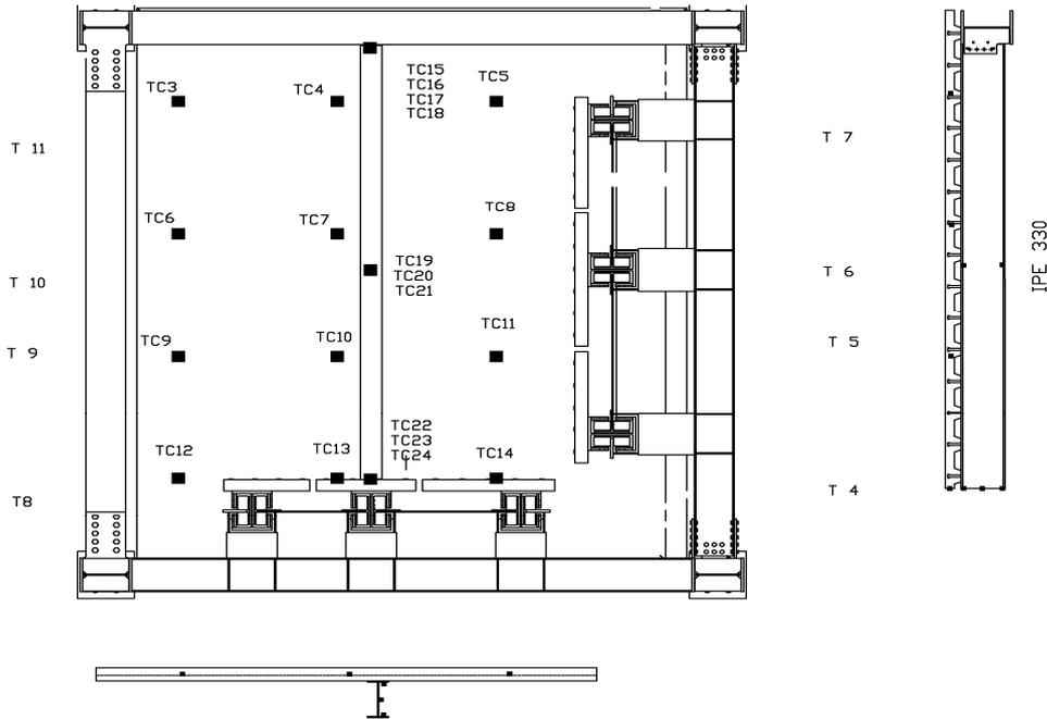
*Figure 5. Location map of the thermo-couples (TC) located inside the furnace and composite floor system.*
