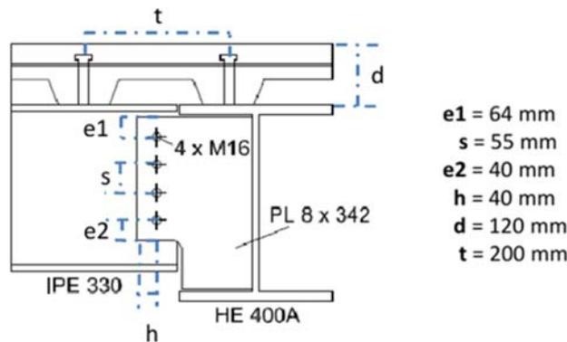
*Figure 3. IPE330 Secondary beam - HEA400 primary beam shear connection detail.*
