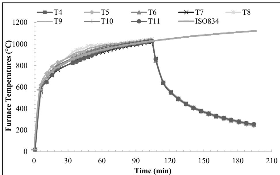
Figure 8. Temperature curves obtained from the different regions of the furnace (see Figure 5).
