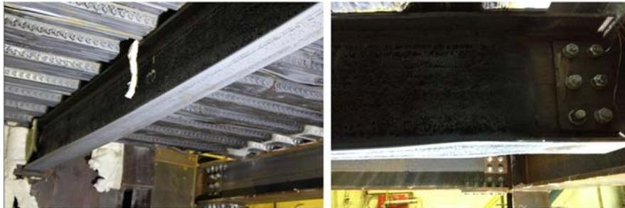
*Figure 12. Deformed shape of the unprotected secondary beam (IPE330) and the steel deck after the test, local buckling on IPE330 beam around the shear connection.*
