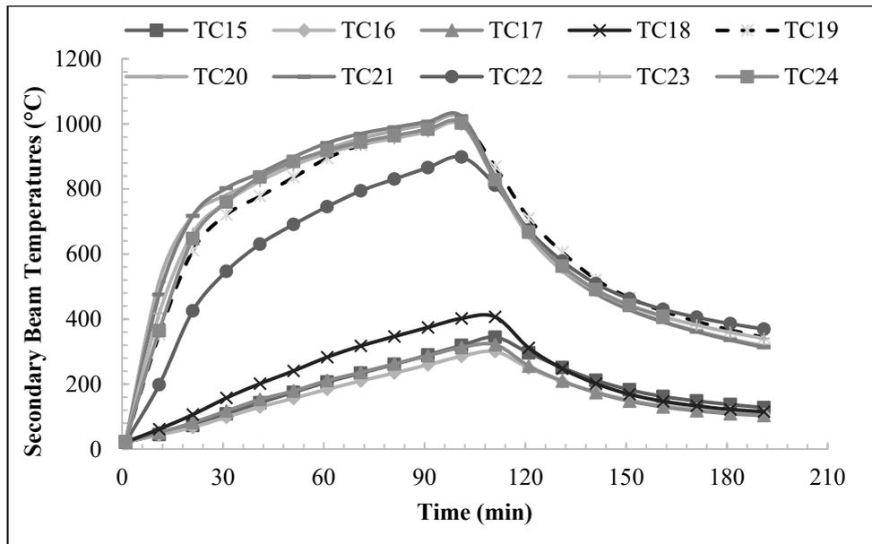
Figure 9. Thermo-couple temperatures on the secondary steel beam IPE330 (see. Fig.5).
