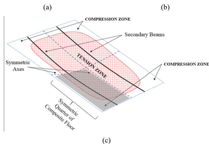
*Figure 13. (a) The top surface of the concrete slab system before the experiment, (b) concrete cracks after the experiment (highlighted in red), (c) illustration of the tensile membrane action.*
