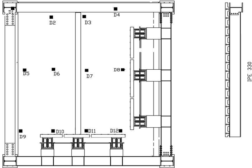
Figure 6. The location map of LVDTs (D1-D12) on the composite floor system.
