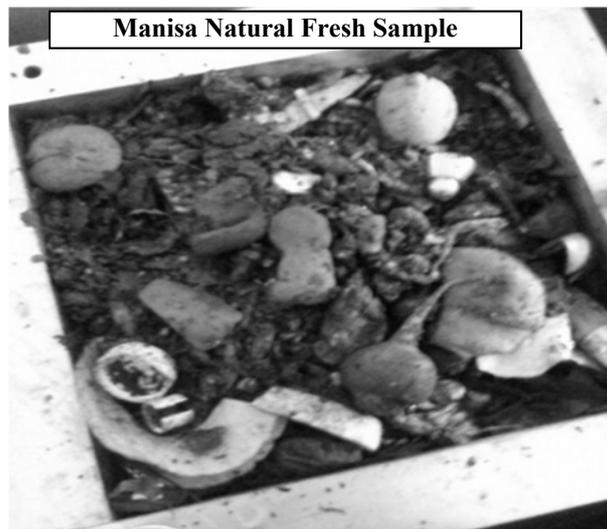
Figure 6. The Manisa natural fresh (M-N-F) sample placed in the shear box
