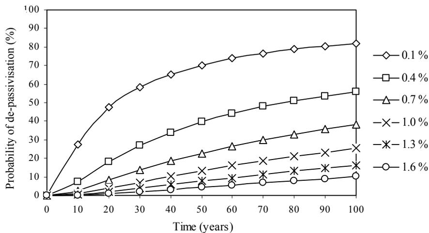
Figure 6. Effect of critical chloride concentration on the probability of de-passivisation
