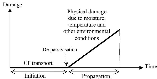
**Figure 1.** Deterioration in structural element due to corrosion of embedded reinforcement
