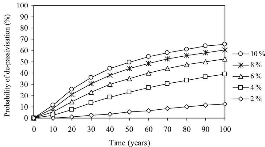
Figure 5. Effect of surface chloride concentration on the probability of de-passivation
