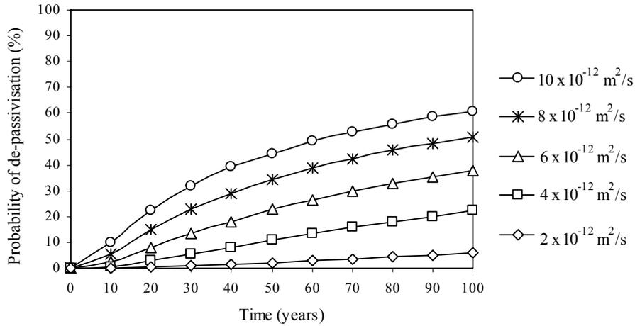
Figure 3. Effect of chloride diffusivity on the probability of de-passivation
