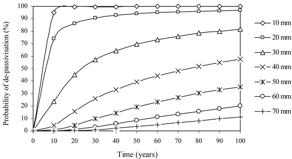
Figure 4. Effect of concrete cover thickness on the probability of de-passivation
